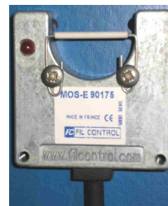
Assembling/Regulation with 2 M4x10 screws
